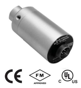
This scanner is used for continuous gas or oil flames. A mechanical shutter in the scanner closes briefly every ten seconds to check for a runaway scanner tube. If a failed tube is detected, the flame safeguard shuts down the system.
